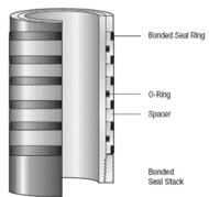
**V-RYTE Seal Stack**—Made up of Viton chevron seals with Teflon and Ryton backup rings, Ryton front-up rings and steel separators.
