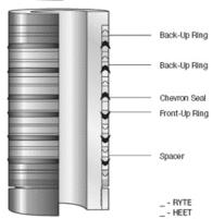
**Debris Barrier Stack**—Made up of Teflon and Ryton backup rings and Ryton front-up rings and steel separators. Used as a wiper to prevent debris from damaging seal stacks when seals are moved after being placed in service.
